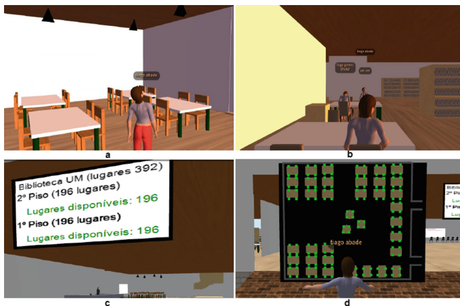
Fig. 2. OpenSimulator representation of the Library: a - ceiling movement sensors (highlighted with triangular markers); b - sitting at a table triggers pressure sensors; c - alphanumeric panel; d - LED panel (Color figure online).
