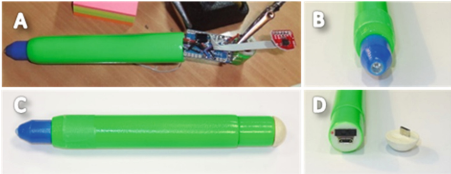
Fig. 2. Augmented pen assembly
