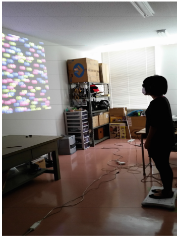
Fig. 2. A scene of the study. The subject stands on a Wii Balance Board to measure body sway with a 2 m viewing distance to the screen. In 3D-movie viewing, subjects wear 3D-glasses.
