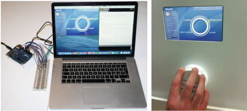
Fig. 4. On the left the Arduino-based board connected to the laptop where programming runs; on the right the final prototype without the soft-touch coating.
