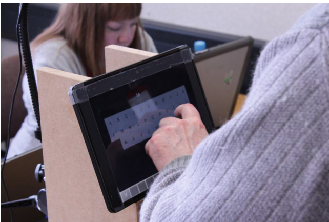
Fig. 3. Touchscreen gestures, such as double-taps and swipes, are unfamiliar to some users, which leads to accidental activation of functions; this picture illustrates a typical problem of knuckles accidentally grazing the screen surface.
