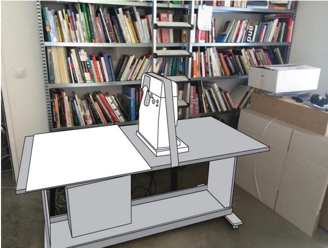
Fig. 1. Tabletop projection setup, where one side of the table (left) has a projection on it emitted from the projector in the middle, affording collaboration in a digital environment (e.g. on presentations), whereas the other side of the table is open for regular, analog work processes (i.e. writing and drawing on paper etc.).
