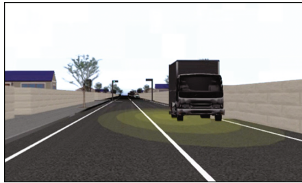
Fig. 10. Visual contents by concentric circles for risky areas in proactive braking situations
