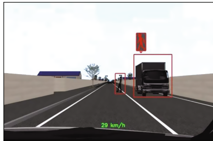
Fig. 5. Visual contents for sharing what the vehicle considers as dangerous [3]. Red rectangles indicates the objects which the intelligent vehicle considers as dangerous. A red sign of pedestrians above the truck indicates potential dangers of pedestrian's running out (Color figure online).
