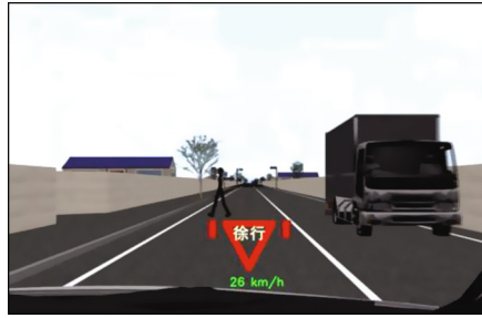
Fig. 7. Visual contents for sharing the state of automated deceleration [3]. A red inverse triangle indicates the deceleration sign in Japan. Red bars beside the inverse triangle indicate the remaining time of deceleration and shorten according to the time (Color figure online).
