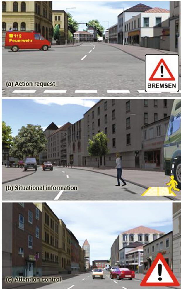
Fig. 3. The three different scenarios with either warning symbols. Scenario (a) action request, scenario (b) situational information, and scenario (c) attention control.
