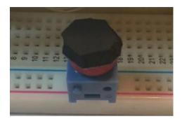
Fig. 4. Button with plain rubber applied
