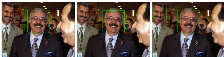
Fig. 3. Face detection applied on images compressed JPEG XR. From left to right the compression ratios are: 1 (reference image), 2 and 100. Image quality is almost identical to JPEG2000. [Image is Part of LFW DB]
