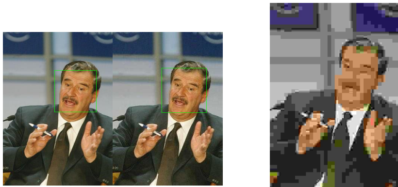
(a) Face detection applied on JPEG images. The left image is the reference image. The image on the right is compressed with a compression ratio of 2. As mentioned, the area where the face is detected differs a little bit from the reference image. [Image is Part of LFW Database] (b) This image was compressed with ratio of 100. Due its high compression leading to blocking artifacts, the detection of a face was not possible. [Image is Part of LFW Database]
