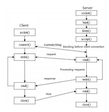
Fig. 2. Working procedure of Socket
