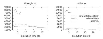
$\textbf{Fig. 4.} \ \, \textbf{Throughput (left)} \ \, \textbf{and rollback count (right)} \ \, \textbf{for the list write-dominated workload:} \ \, \textbf{dynamic thread allocation}$
