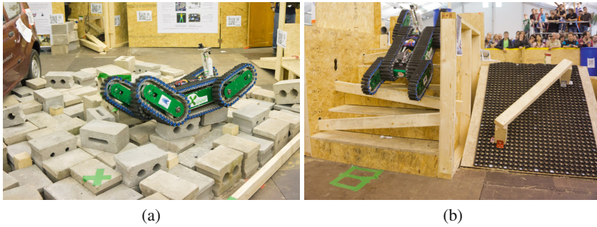
Fig. 2. New mobility apparatuses at the RoboCup 2013 in Eindhoven, Netherlands: (a) Stepfield made of concrete blocks. (b) Occluded stair and ramp apparatuses.
