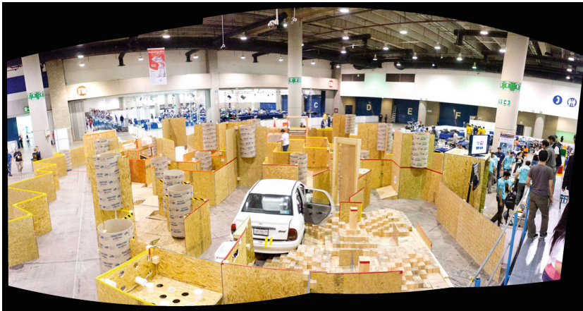
Fig. 1. Overview of a RoboCup rescue arena, composed of standardized test elements, organized in a maze. This image depicts a typical International Championship arena (in this case from the 2012 competition in Mexico City)(Color figure online).
