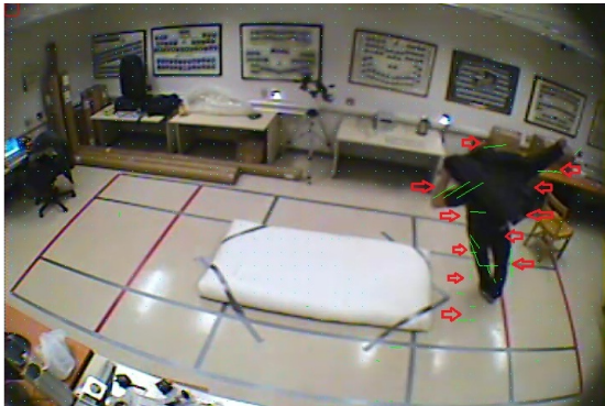
Fig. 1. Motion vectors extracted from a frame of the fall dataset. The red arrows highlight the regions in which the motion field exhibits strong disorder.
