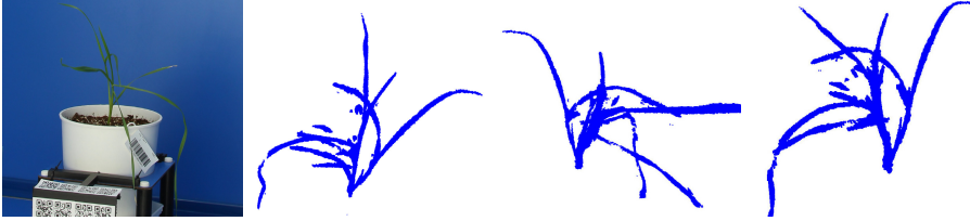
Fig. 2. A visual hull reconstruction illustrating the spurious shapes beyond the true plant reconstruction which are inherent to the visual hull
