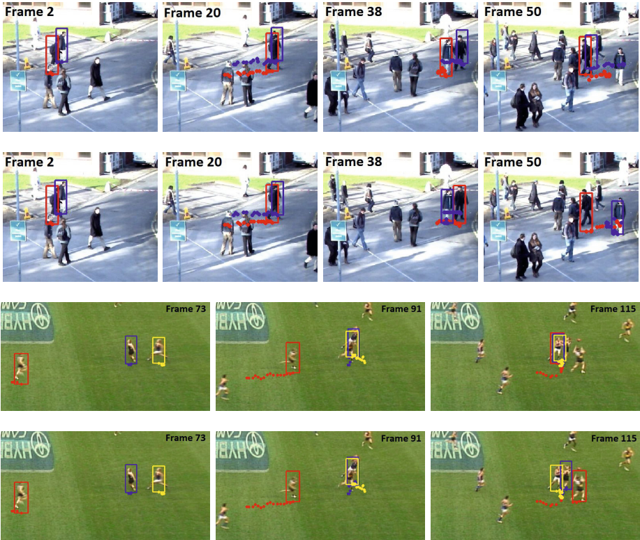
Fig. 3. Visual trackers without (1 st and 3 rd rows) and with (2 nd and 4 th rows) local data association. See text for details.
