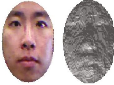
Fig. 1. Examples of 2D (left) and 3D (right) cropped face images obtained with the Microsoft Kinect sensor after preprocessing
