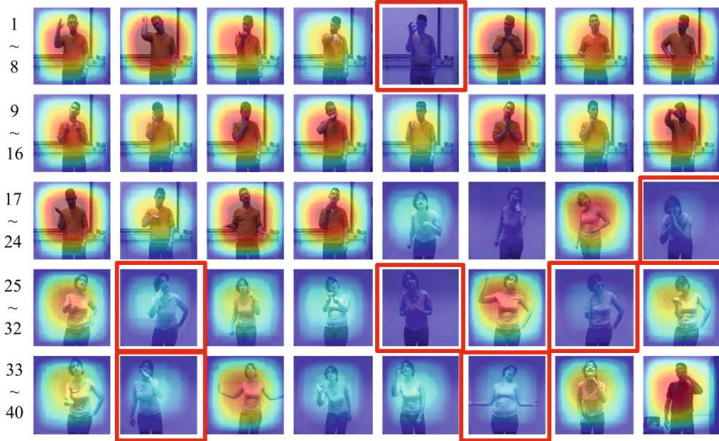
Fig. 6. The 2D heat maps of the dominant positions of the first 40 gesture segments in the testing dataset. Red rectangles mean the mis-classified gesture segments. Red indicates high frequency and blue indicates low frequency.(best viewed in color)
