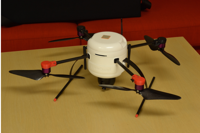
Fig. 1. LinkQuad platform with the color camera sensor module
