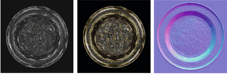
Fig. 13. (left) Specular quotient = ratio of specular/diffuse intensities; (centre) specular colour; (right) Specular direction vectors in false colour
