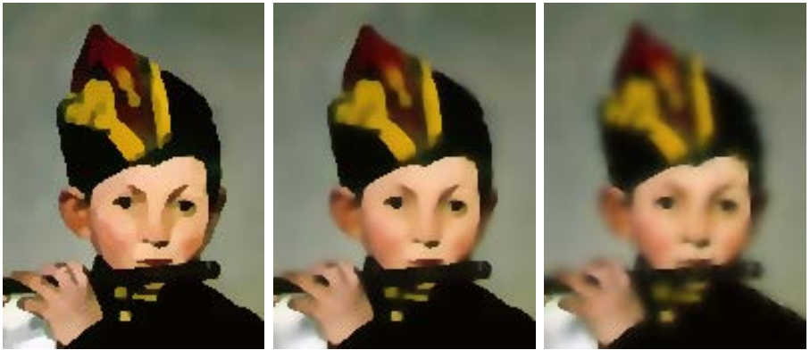
Fig. 6. Matrix-valued M-smoother with exponent p and 5 iterations. Left. IAMS with p = 1 identical to IAMF. Middle. IAMS with p = 2 , i.e. the image shows an amoeba-based arithmetic mean. Right column. IAMS with p = 5 .
