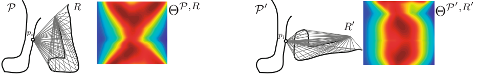
Fig. 2. (best seen in color). Extended OCTAR descriptor for contours spatial configuration. The same two contours under different configurations have different descriptor.
