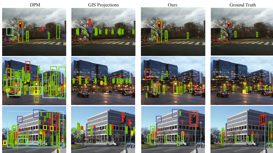
Fig. 5. Sample object detection results. For each sample, the detections found by DPM and our method, along with the GIS projections and the ground truth are shown. Our method significantly improved the results in these challenging urban-area images.
