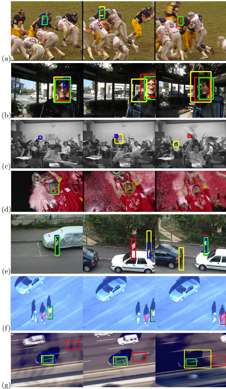
Fig. 5. Tracking results on (a) Football1, (b) Trellis, (c) Freeman4, (d) Soccer, (e) Woman sequences from the benchmark dataset [48], and (f) Pedestrian2, (g) Car chase sequences from the TLD dataset [24]. Green: Our result, Red: Struck, Yellow: SPLTT, Blue: TLD. See text for details. (Best viewed in pdf.)
