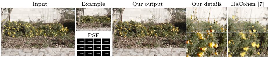
Fig. 7. Test image from HaCohen et al. [7] with spatially varying PSF estimates. Our approach is highly competitive without requiring dense correspondence.
