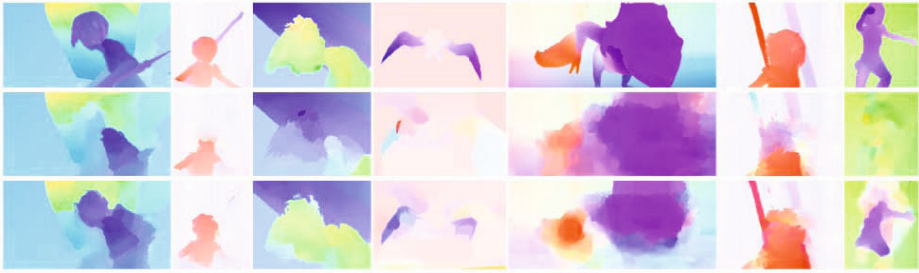
Fig. 8. Results on the “final” training sequences. Top row: Ground truth. Middle row: Results with Classic+NL. Bottom row: Results with Channel-Flow and the two additions (C-Flow+I+C).
