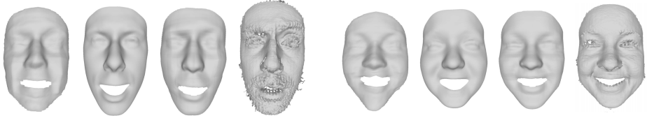
Fig. 5. Reconstruction examples for noisy scans in different expressions. Left block: fear expression. Right block: happy expression. Each block, from left to right: local multiple PCA [8], global multilinear [7], proposed ( \rho_S = 100 ), input data.
