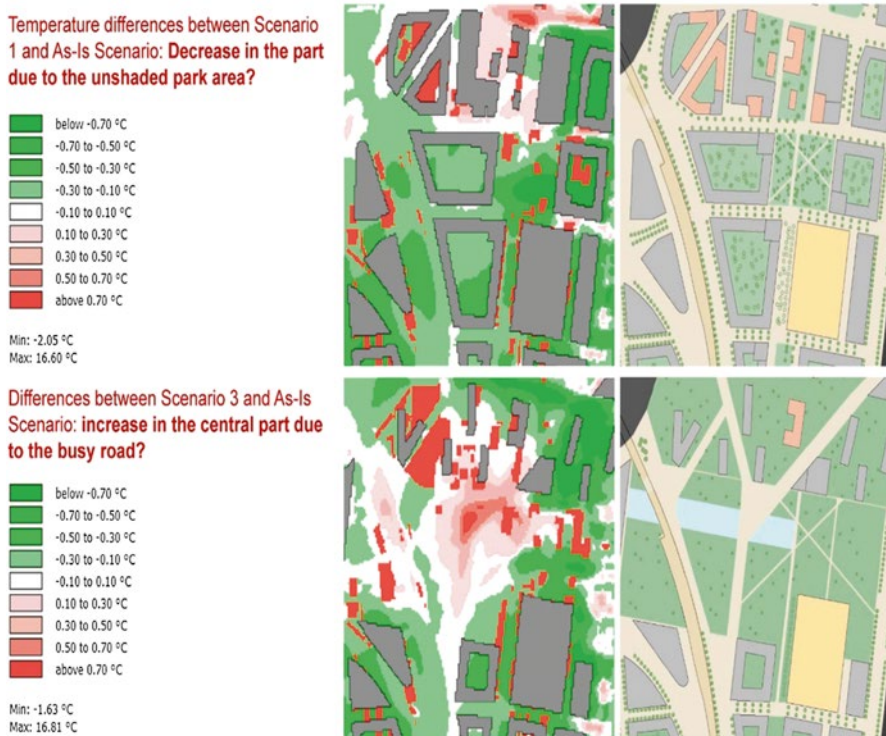
Fig. 14.30 The cooling effect of green roofs is negligible
