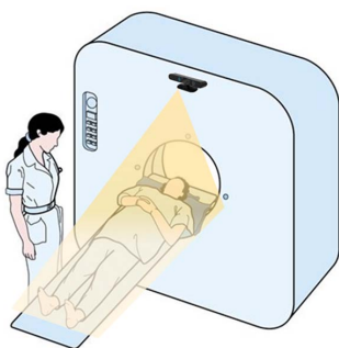
Fig. 1. Structured Light Depth Sensor mounted on top of a CT Scanner
