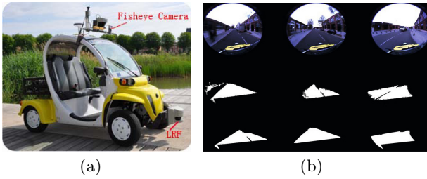
Fig. 4. (a) The configuration of the used experimental platform (b) Experimental results. The images of the first row are original images, the second row are results obtained using the approach proposed in paper [6], the third are the results obtained by the proposed method in this paper.
