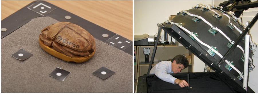
Fig. 2. (left) Photogrammetric imaging setup with scarab on target board; (right) positioning the scarab on the baseboard of the UCL dome
