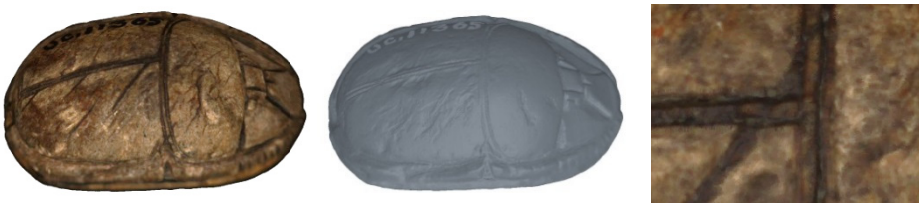
Fig. 6. (left) The 3D reconstruction from photometric stereo produced a very dense point cloud with outstanding detail of surface features, which enabled the researcher to interpret the object
