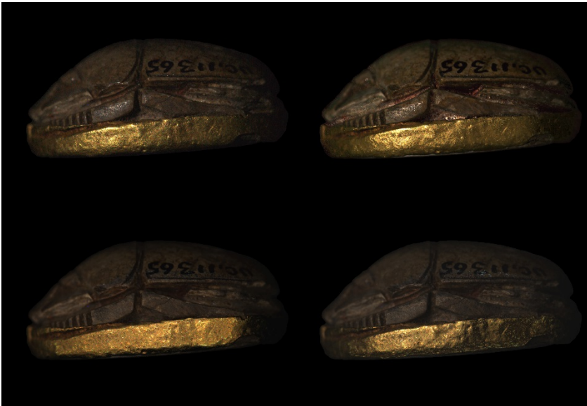
Fig. 3. Screenshots from the custom software viewer showing specularly of gold in four representations of the left side of the scarab: (top left) original image; (bottom left) PTM model; (bottom right) hemispherical harmonics (HSH) model; (top right) Lorentzian specular model
