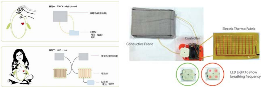
Fig. 3. Two modes of intimacy. The electronic circuits and the smart textiles used.
