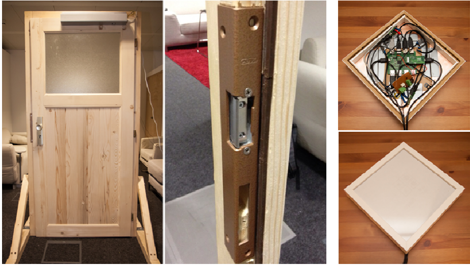
Fig. 5. Overview of the prototype system. Left - door full view. Middle - door close-up of locking mechanism. Right - control unit open and closed view.
