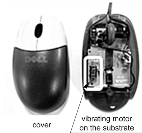
Fig. 3. Vibration mouse presenting vibration rhythm
