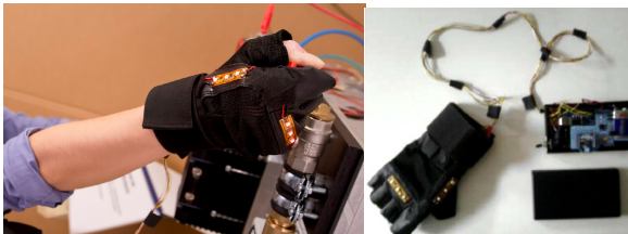
Fig. 1. Warning glove with multimodal devices (left) and glove with Arduino microcontroller and XBee receiver (right)
