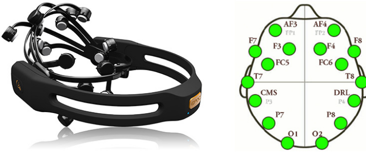
Fig. 1. The Emotiv EPOC and the electrodes location
