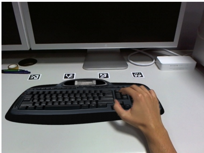
Fig. 5. Compositing and final result. The original real background shown in Fig. 3 is composited according to the disparity map of the scene enabling a correct visualization and a meaningful interaction (note that hand's casted shadow is not currently handled by the proposed method).
