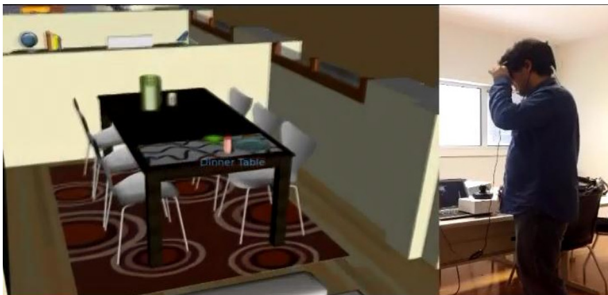
Fig. 3. User selecting an object (dinner table) by head orientation (HOS) while immersed in a VE created with pSIVE
