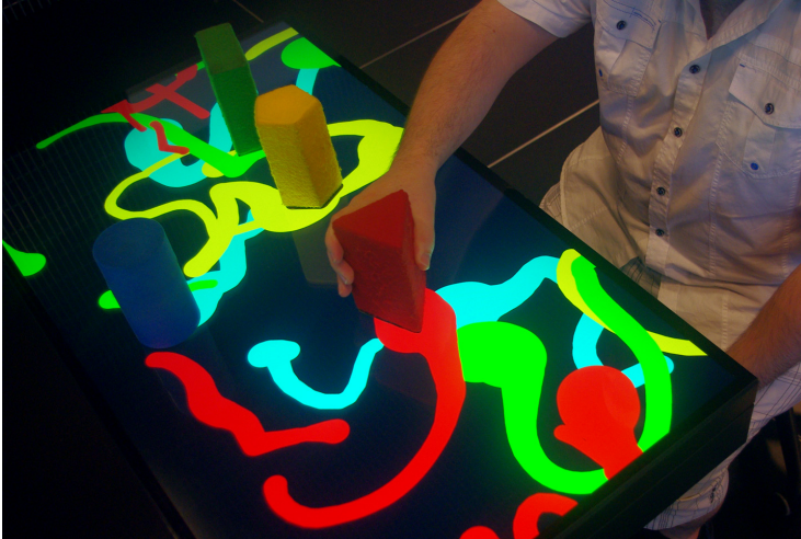
Fig. 2. An individual using the Elements system explores the functions of several soft graspable tangible user interfaces to draw and paint digitally
