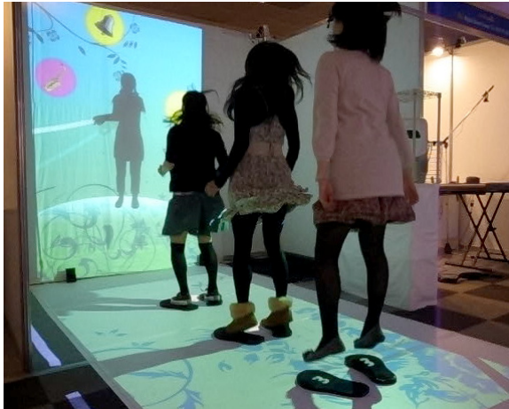
Fig. 1. The Group Jump Rope system. A virtual rope is projected on two screens at the front and the floor. Participants jump when the rope passes under their feet.
