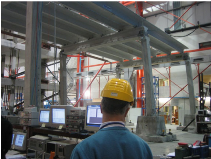
Fig. 4.25 The ultimate drift of 8 % (top displacement equal to 40 cm) was observed in PRECAST full-scale test
