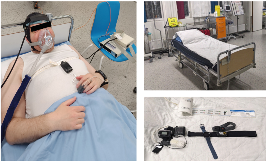
Fig. 2. We put several devices on the subject and the one on the forehead was our fNIRS device (left). Measurement environment at Clinical Skills Centre Knoppi and some sensors (right)
