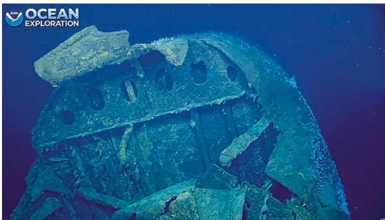
Fig. 9.5 ROV image of the broken stern end of Bloody Marsh at the jointery between the engine room and cargo tanks (NOAA Ocean Exploration)
