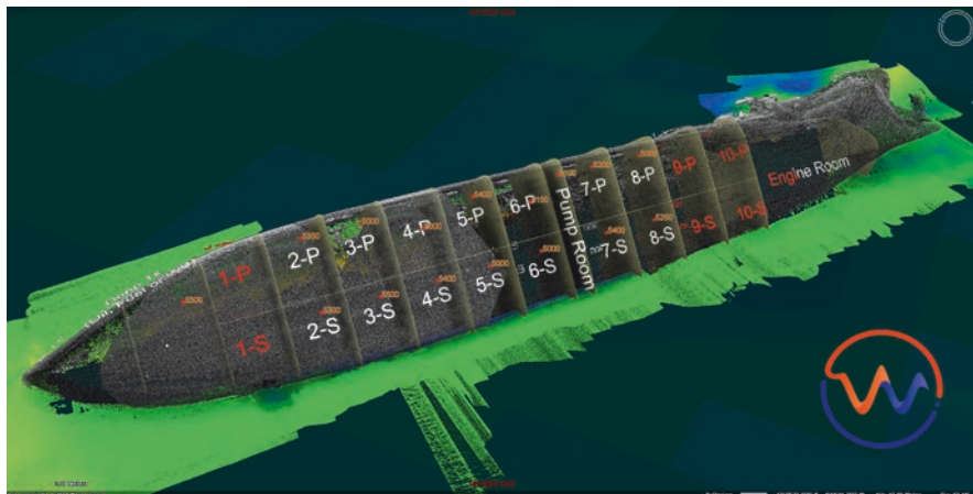
Fig. 11.4 NBS sampling regime and results overlaid on the integrated data model of the Derbent
