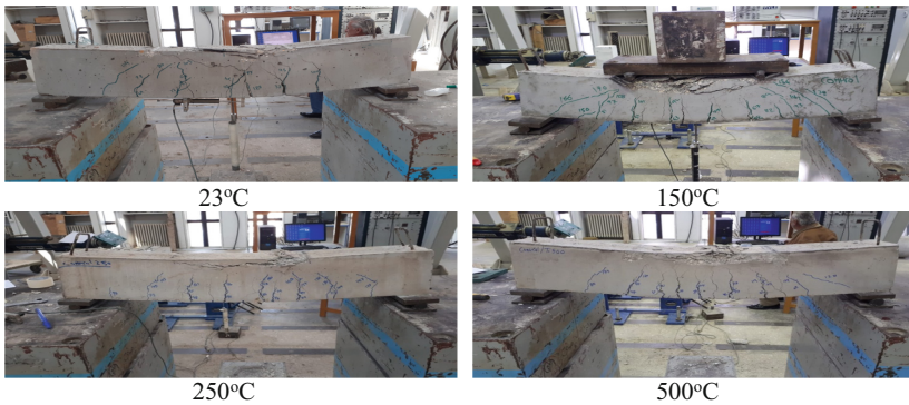
Fig. 4. The effect of temperature on the failure mode of the control specimen.
