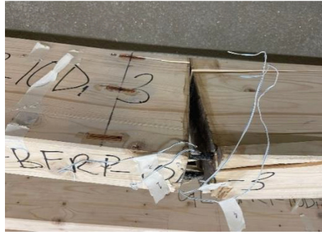
(a) 10 – D1 – 3: Debonding; splitting of timber along the bar at compression zone; splitting of timber at tension zone at soffit and size of beam
