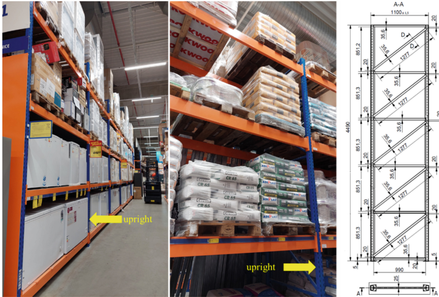
Fig. 1. Pallet rack storage system in a typical warehouse in Romania and the dimensions of the vertical upright frame.
