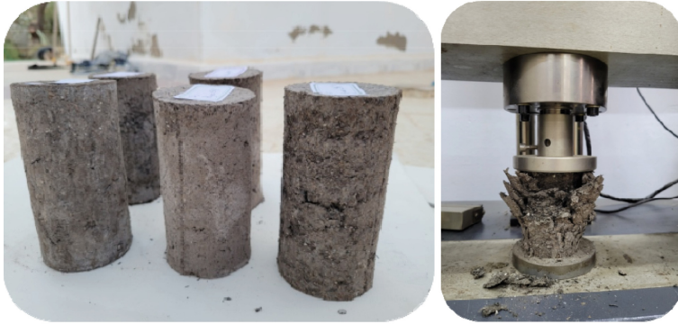
Fig. 4. Specimens with a diameter of 70 mm and a height of 140 mm, featuring various percentages of Ulva for the compression test (taken by the author).
