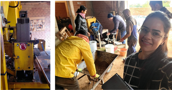
Fig. 8. Production of blocks using Ulva at a local company ‘SOIB’.
