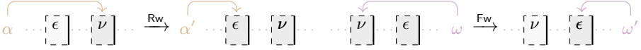
Fig. 3. Schematic depictions of the rewind and forward rewrite rule, focusing on a single location, where the initial/final view points to \nu before and points to \epsilon after. The messages \nu and \epsilon may coincide, dovetail, or be separated. Left: The initial view \alpha is “rewound” to \alpha' . Right: The final view \omega is “forwarded” to \omega' .
