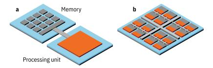
Fig. 1 a von Neumann architecture and bottleneck between memory and processing unit and  $\mathbf{b}$  neuromorphic chip architecture
