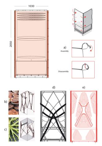
Fig. 2. Biomimetic design development of the side wall of the portable toilet.
