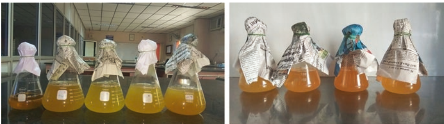
Fig. 7.1 Preparation of bacterial solution: (a) Subcultured Bacillus subtilis bacterial solution, (b) Subcultured Bacillus cereus bacterial solution
