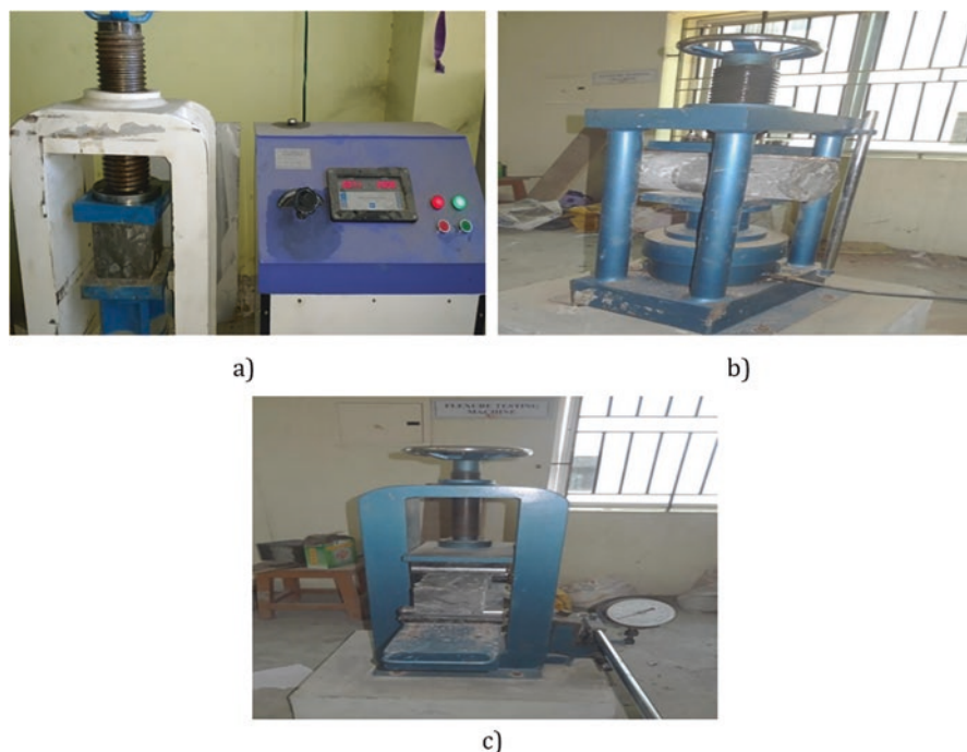
Fig. 7.3 Experimental test setups: (a) Compressive strength test, (b) Splitting tensile strength test, (c) Flexural strength test
