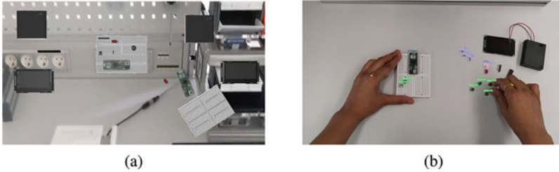
Fig. 3 (a) Synthetic image for assembly objects, (b) object detection on a video captured from HoloLens2 for the corresponding real objects
