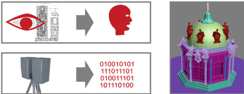
Fig. 2.11 Schematic reconstruction (upper left) versus digitization (lower left) workflow, both resulting in a virtual 3D model (right) (Images: Münster, except right: Rainer Uhlemann, lightframe fx)
